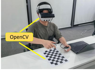
(a) Camera-Chessboard Calibration
